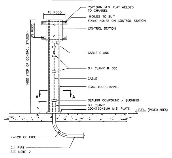
$A = \begin{cases} 150 \text{ MM (MIN.) FOR INDOOR LOCATION} \\ 300 \text{ MM (MIN.) FOR OUTDOOR LOCATION} \end{cases}$
